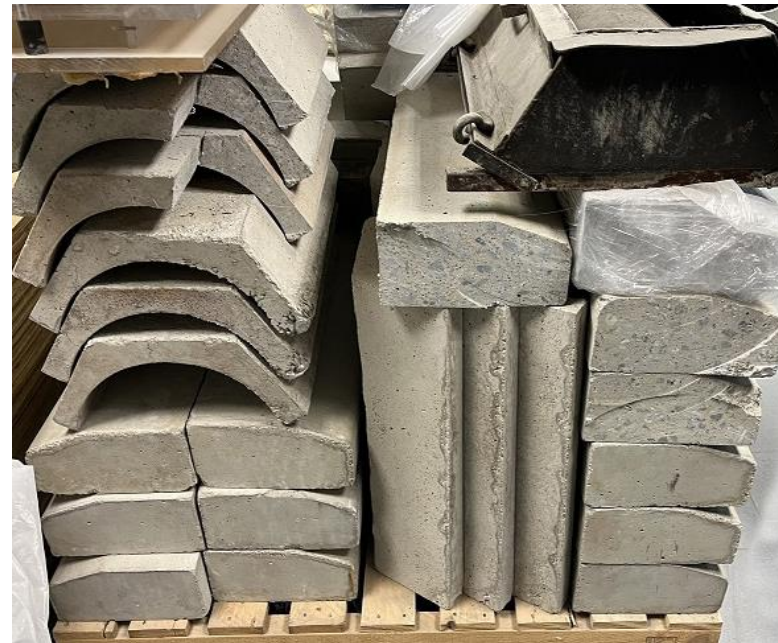
Concrete with 30% recycled plastic moulded into drain channels & footpath kerbs
