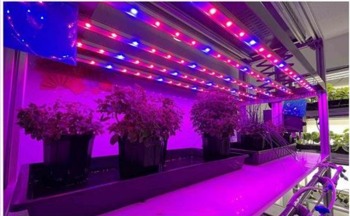
Measuring plant growth performance & yield under tailor made LED light spectrum
