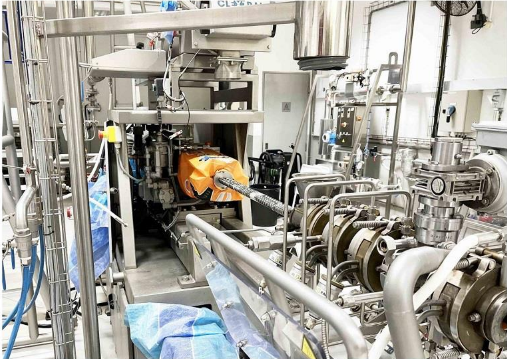
Front view of the extrusion barrel and pellets separators
