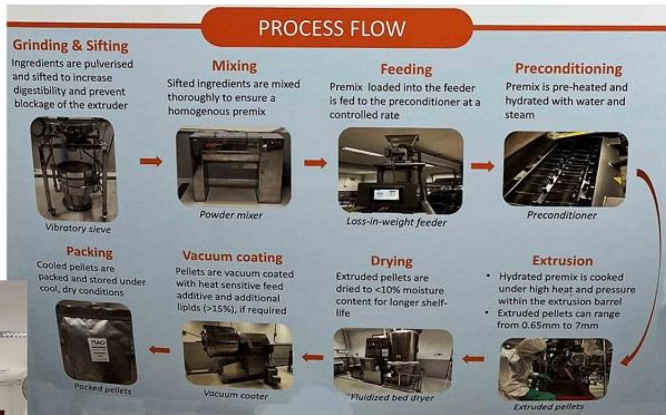
MAC's pilot feedmill process flow chart
