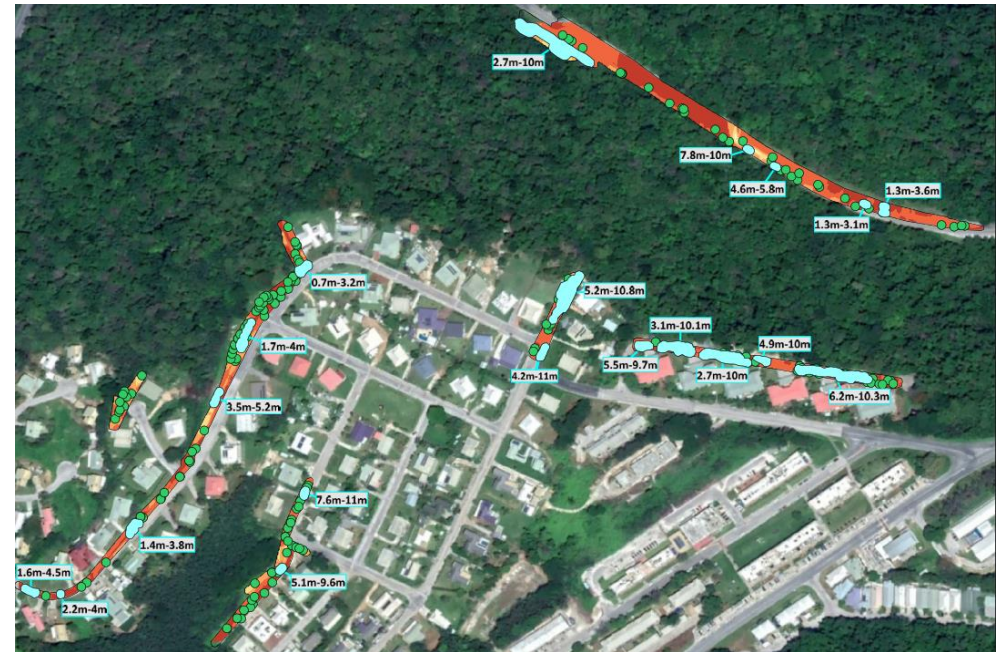
Figure 2 – MNG interpreted karst/voids indicating depth below ground level
