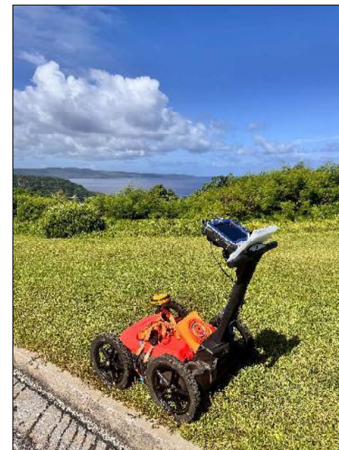
Figure 2: GPR data acquisition using the GSSI 350HS system on site.
